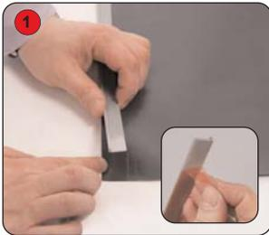
Slide the plastic insert from the cassette & adhere to the **back** of the graphic.
